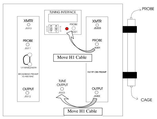
9. When completed, change the CHAN channel back to 0 by pressing the - key once. The TUNING INTERFACE readout should blank, and the red light should start blinking.
