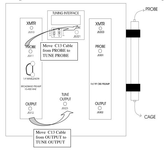
Tuning Interface Module. Arrows indicate where cables are moved for <sup>13</sup>C Tuning.
